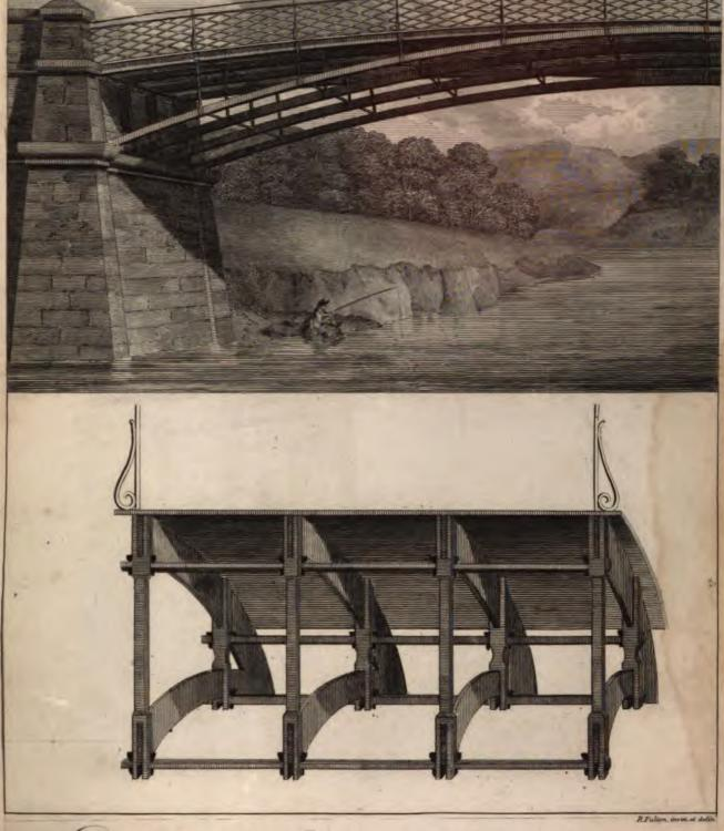
Design for an Fron Bridge Scale I Inch to 10 Feet. tion Shows the Rils and Braces Scale I Inch to 4 Feet.
